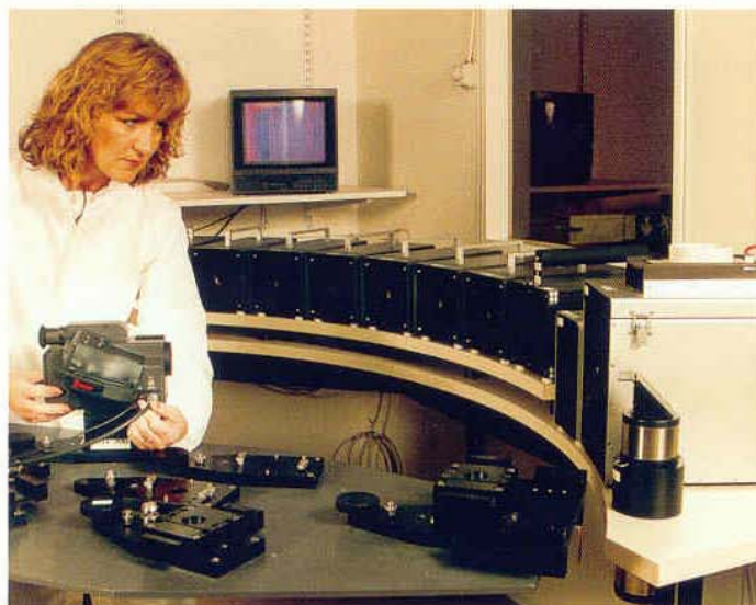
Calibration room. All cameras are individually calibrated.
